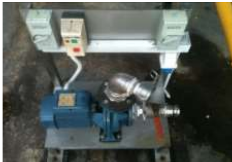
Portable trolley for filling IBCs with Magflow's
