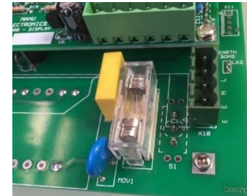
Fuse RHS rear of PCB)
