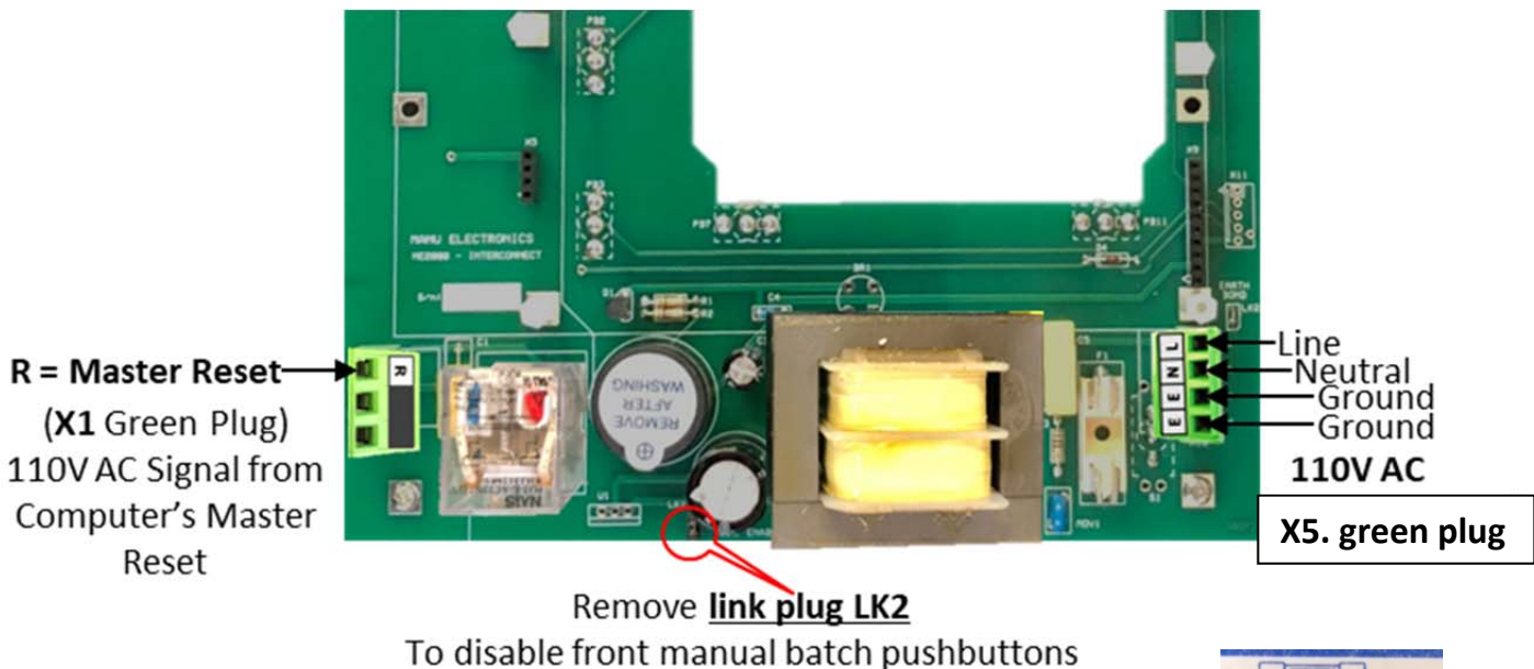
Figure 1. Motherboard Wiring Diagram, X1 and X5 plugs
