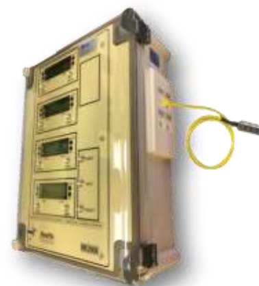
ME2008 8-channel unit, opened, with external 8CAT5e Programmer
