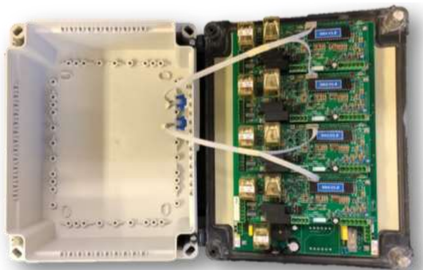
ME2008 8-channel unit, opened, with external 8CAT5e Programmer
